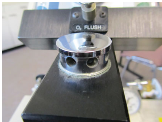
Figure 5.23 Air entrainment valve.
